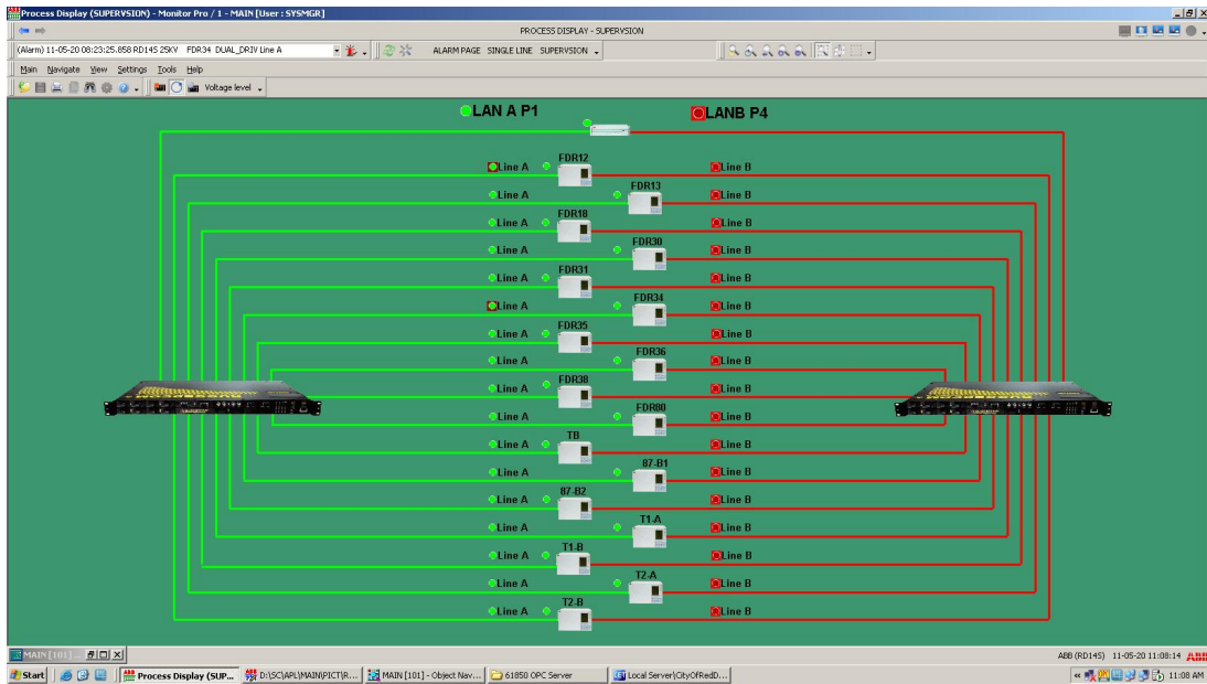
Figure 5 - HMI Communications Supervision Page
