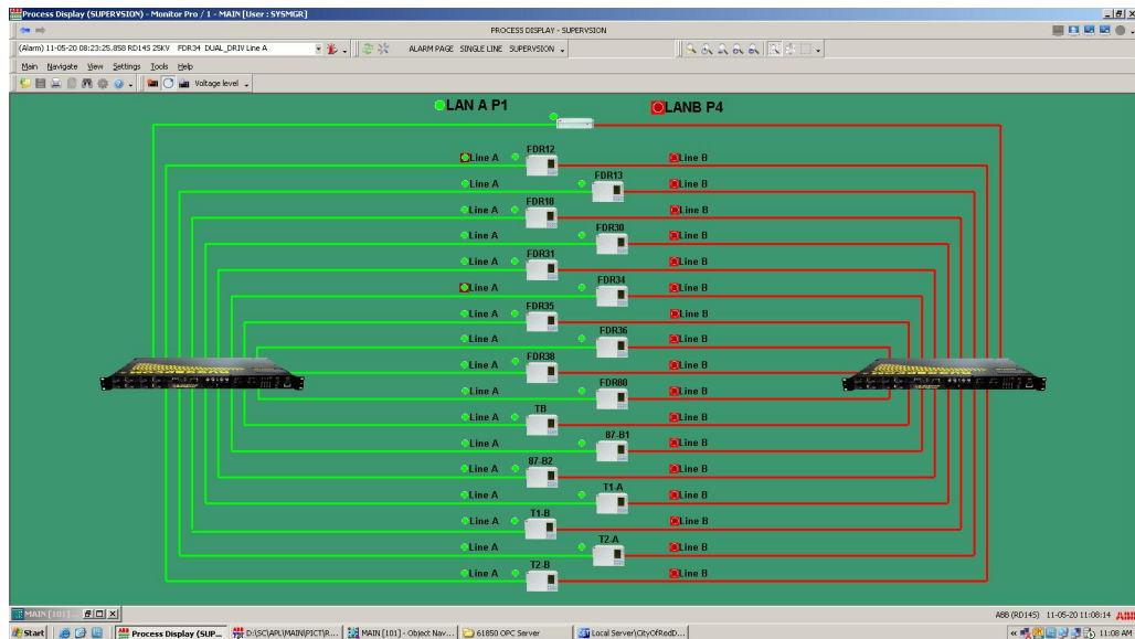
Figure 9 - HMI Communications Supervision Page
