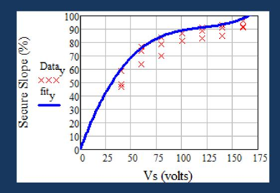
• Fitted curve:  $k_{max} = 0.000046Vs^3 - 0.0166Vs^2 + 2.09Vs$  for  $V_s \le 160$
